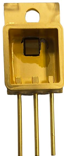
Figure 1. TO-254 Package with SiC integration for preliminary work
